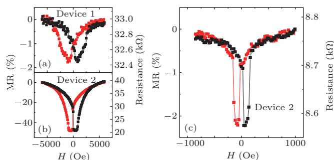
**Fig. 8.** MR curves of OSV devices fabricated on (a) as-grown LSMO film, (b) optimally annealed LSMO film, respectively, at 10 K. (c) Room temperature MR curve for OSV fabricated on optimally annealed LSMO film.<sup>[30]</sup>
