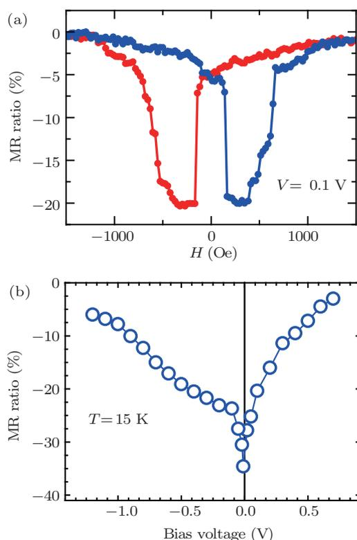
**Fig. 9.** (a) MR curve for OSV device of LSMO (100 nm) / Alq<sub>3</sub>(25 nm) / Co(20 nm) / Al(15 nm) measured at 15 K with a bias voltage of 0.1 V. (b) The MR as a function of the bias voltage measured at 15 K.
