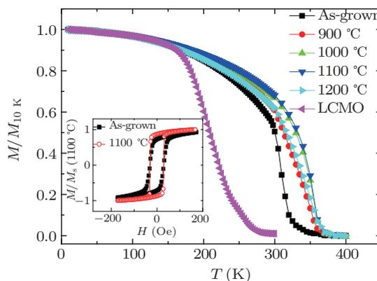
Fig. 4. Temperature dependent normalized magnetization of LSMO films annealed at different temperatures.<sup>[30]</sup>
