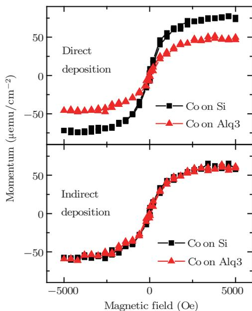
**Fig. 7.** Room-temperature magnetization hysteresis loops measured by vibrating sample magnetometer (VSM) for Co films on Alq<sub>3</sub> and Si deposited by direct and indirect deposition methods, respectively.<sup>[37]</sup>
