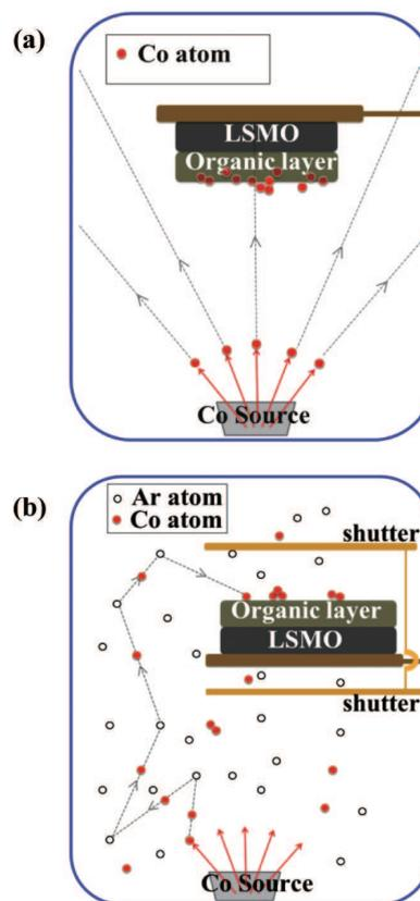
Fig. 6. Schematic diagrams of (a) direct deposition and (b) indirect deposition.<sup>[37]</sup>
