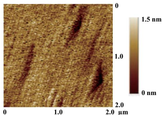
Fig. 5. AFM image of Alq<sub>3</sub> (50 nm) grown on SrTiO<sub>3</sub>.
