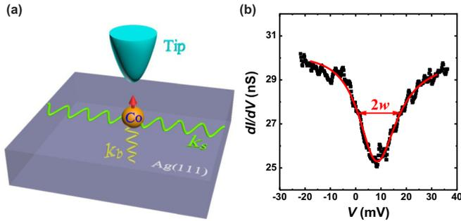
FIG. 1. (a) Sketch of the Kondo resonance measurement with a STM in the presence of both bulk and surface states. (b) Typical Kondo resonance curve measured for a single Co adatom on a wide Ag(111) terrace at 4.7 K ( $V_b = 50$  mV and  $I = 1$  nA). Red curve is the fitting that utilizes Eq. (1).
