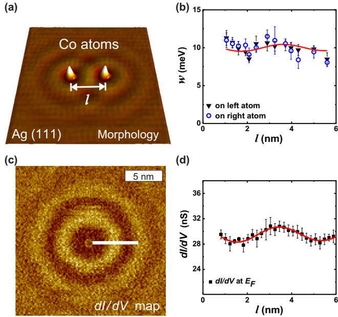
FIG. 3. (a) Topographic view of two Co adatoms separated with distance  $l$  and on a wide Ag(111) terrace. (b)  $l$ -dependent Kondo resonance width obtained on top of both adatoms. (c) The experimentally obtained  $dI/dV$  mapping at  $E_F$  ( $-0.1$  meV) within the vicinity of a single Co adatom. (d) Line profile of  $dI/dV$  as marked in (c). Red curves are fittings (see text). In all measurements,  $V_b = 50$  mV and  $I = 1$  nA.
