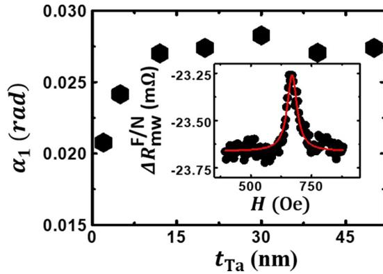
FIG. 4. In-plane precession angle as a function of Ta thickness. The inset shows a typical microwave photoresistance signal used for the estimation of the in-plane precession angle. The signal was obtained with  $\alpha_0 = 90^\circ$  and  $f = 10$  GHz for Ta (20)/CoFeB (10).
