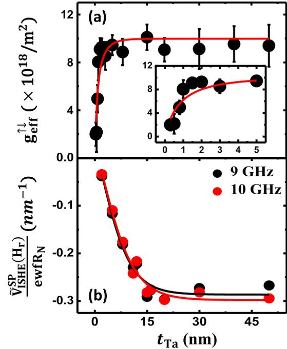
FIG. 5. (a) Ta thickness dependence of the effective spin mixing conductance. The solid line is the fit according to Eq. (1). The inset shows the effective spin mixing conductance as a function of Ta thickness in the range 0–5 nm. (b) Ta thickness dependence of ISHE signal measured at 9 GHz (black circle) and 10 GHz (red circle). The solid lines are the fits utilizing Eq. (2).
