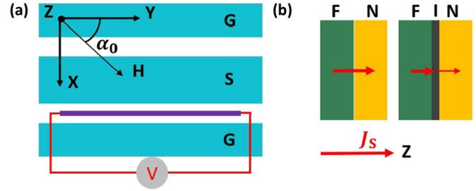
FIG. 1. (a) Schematic illustration of the experimental setup for the spin pumping induced ISHE voltage measurement. The Ta/CoFeB bilayer is placed in the middle of the gap between the ground (G) and signal (S) lines of a coplanar waveguide. (b) Schematic illustration of spin current transmission across the interface (I) between ferromagnetic (F) and normal (N) layers without considering interface spin loss (left) and with the interface spin loss (right).
