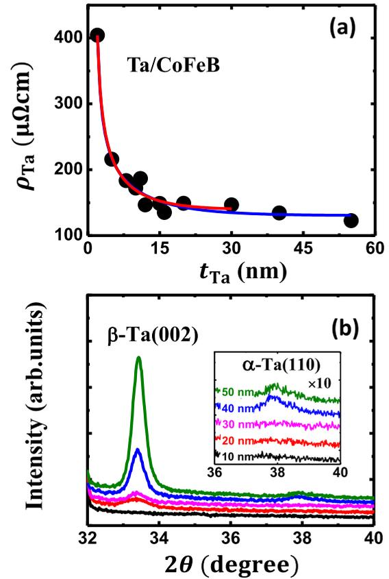
FIG. 3. (a) The Ta thickness-dependent resistivity. Symbols are the experimental data, and the lines is a fit using the Fuchs-Sondheimer model. (b)  $\theta$ - $2\theta$  XRD scan of Ta (10, 20, 30, 40, and 50 nm) films deposited on GaAs substrates. The inset shows the amplified view.
