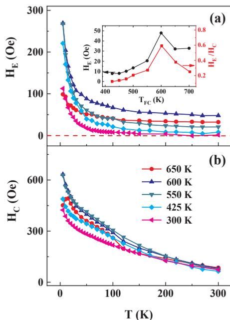
Fig. 6. Temperature dependences of  $H_E$  and  $H_C$  for sample 1 after being field cooled under  $H_{FC} = 0.5$  T with various  $T_{FC}$ . The inset shows the  $T_{FC}$  dependences of  $H_E$  and  $H_E/H_C$  measured at RT for sample 1.
