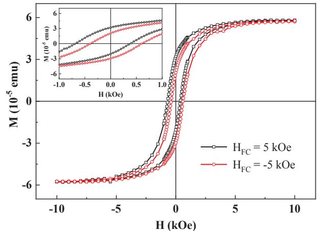
Fig. 3. The  $M$ - $H$  loops measured at 5 K after sample 2 was field cooled from 300 K to 5 K under  $H_{\text{FC}} = \pm 0.5$  T. The insets are the corresponding enlarge views of the  $M$ - $H$  loops at low- $H$  region.
