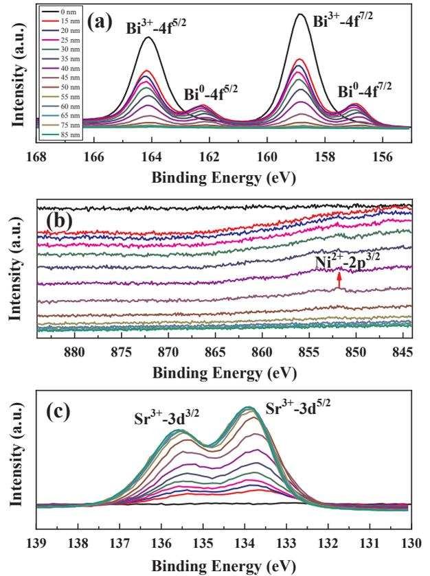
Fig. 2. The depth profile XPS spectra for (a) Bi-4f, (b) Ni-2p and (c) Sr-3d for sample 1. The red arrow in (b) is indication of the peak for  $\text{Ni}^{2+}\text{-2p}^{3/2}$ .
