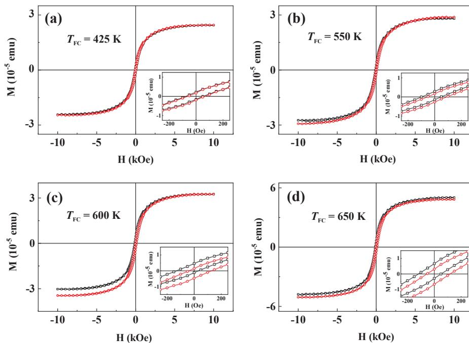
Fig. 5.  $M$ - $H$  loops measured at RT for sample 1 cooled to RT under  $H_{FC} = 0.5$  T (in black) and  $-0.5$  T (in red) with  $T_{FC}$  equal to 425 K (a), 550 K (b), 600 K (c) and 650 K (d), respectively. The insets show the corresponding enlarged views of  $M$ - $H$  loops at low- $H$  region.
