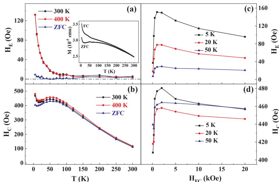
Fig. 4. (a) Temperature dependences of  $H_E$  for ZFC and FC ( $H_{FC} = 0.5$  T,  $T_{FC} = 300$  K and 400 K) for sample 2. The inset is the ZFC-FC  $M$ - $T$  curves measured under 0.5 T for sample 2. (b) Temperature dependences of  $H_C$  for ZFC and FC ( $H_{FC} = 0.5$  T,  $T_{FC} = 300$  K and 400 K) for sample 2.  $H_{FC}$  dependences of  $H_E$  (c) and  $H_C$  (d) measured at  $T = 5$  K, 20 K and 50 K for sample 2.
