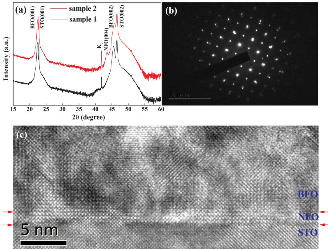
**Fig. 1.** (a) XRD patterns for sample 1 and sample 2. (b) The SAED pattern for sample 1. (c) The HRTEM image for sample 1. The red arrows are indications of the STO-NFO and NFO-BFO interfaces.
