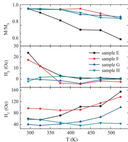
**Fig. 4.** Annealing temperature ( $T$ ) dependences of (a)  $M/M_S$ , (b)  $H_C$  and (c)  $H_E$  for samples E and G cooled under 1000 Oe and for samples F and H cooled under  $-1000$  Oe by conventional heat treatments.
