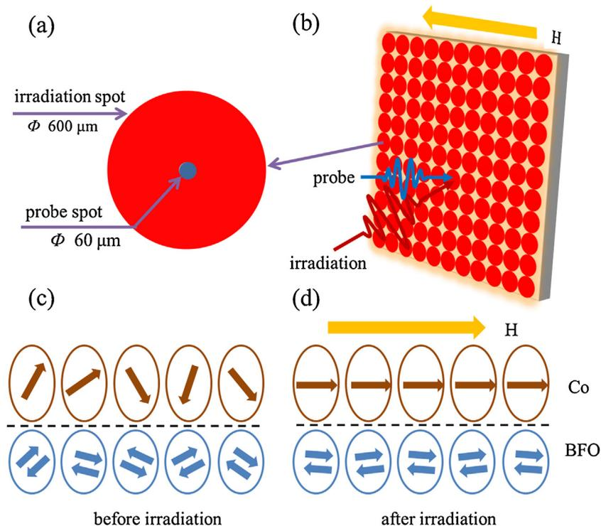
**Fig. 1.** Schematic illustration for laser irradiation and MOKE detection on a small single spot (a) and a whole sample (b). Schematic illustration for the expected alignment of interfacial FM and AFM domains before (c) and after (d) irradiation under a magnetic field.
