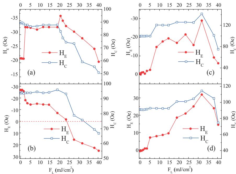
**Fig. 3.** The laser fluence ( $F_L$ ) dependences of  $H_E$  and  $H_C$  for samples A and C irradiated under 1000 Oe ((a) and (c)), and for samples B and D irradiated under  $-1000$  Oe ((b) and (c)). Arrows and dotted lines are guide to eyes.
