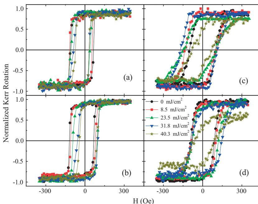
Fig. 2. *M-H* loops measured after different laser fluence irradiation under 1000 Oe for samples A and C ((a) and (c)), and under -1000 Oe for samples B and D ((b) and (d)).
