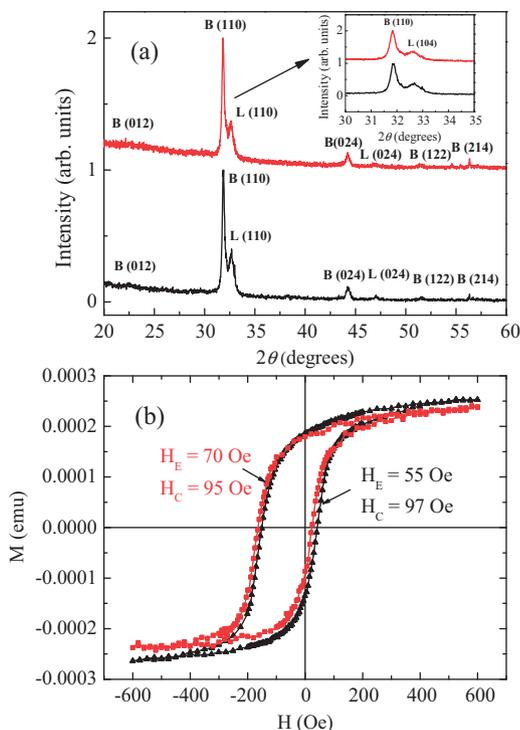
**Fig. 5.** XRD patterns (a) and  $M-H$  loops (b) obtained for sample J before and after laser annealing on the whole sample under 1000 Oe. The enlarged XRD patterns around  $2\theta = 32^\circ$  are shown in the inset of (a). 'B' and 'L' denote  $\text{BiFeO}_3$  and  $\text{LaNiO}_3$ , respectively.
